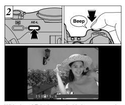
With the "AE-L" button held down, press the shutter button down halfway to focus the shot and then compose the shot again.
